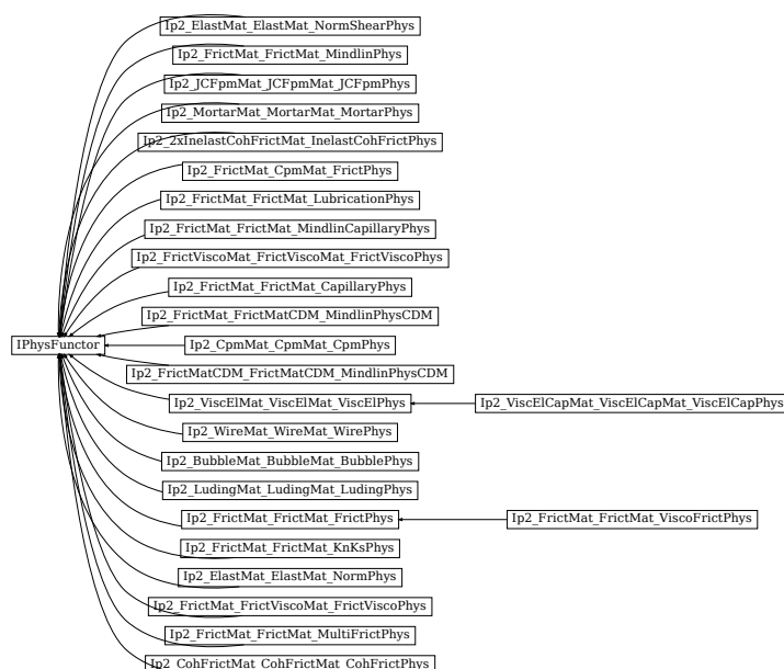
Fig. 35: Inheritance graph of IPhysFunctor. See also: Ip2_2xInelastCohFrictMat_InelastCohFrictPhys , Ip2_BubbleMat_BubbleMat_BubblePhys , Ip2_CohFrictMat_CohFrictMat_CohFrictPhys , Ip2_CpmMat_CpmMat_CpmPhys , Ip2_ElastMat_ElastMat_NormPhys , Ip2_ElastMat_ElastMat_NormShearPhys , Ip2_FrictMatCDM_FrictMatCDM_MindlinPhysCDM , Ip2_FrictMat_CpmMat_FrictPhys , Ip2_FrictMat_FrictMatCDM_MindlinPhysCDM , Ip2_FrictMat_FrictMat_CapillaryPhys , Ip2_FrictMat_FrictMat_FrictPhys , Ip2_FrictMat_FrictMat_KnksPhys , Ip2_FrictMat_FrictMat_LubricationPhys , Ip2_FrictMat_FrictMat_MindlinCapillaryPhys , Ip2_FrictMat_FrictMat_MindlinPhys , Ip2_FrictMat_FrictMat_MultiFrictPhys , Ip2_FrictMat_FrictMat_ViscoFrictPhys , Ip2_FrictMat_FrictViscoMat_FrictViscoPhys , Ip2_FrictViscoMat_FrictViscoMat_FrictViscoPhys , Ip2_JCFpmMat_JCFpmMat_JCFpmPhys , Ip2_LudingMat_LudingMat_LudingPhys , Ip2_MortarMat_MortarMat_MortarPhys , Ip2_ViscElCapMat_ViscElCapMat_ViscElCapPhys , Ip2_ViscElMat_ViscElMat_ViscElPhys , Ip2_WireMat_WireMat_WirePhys .
