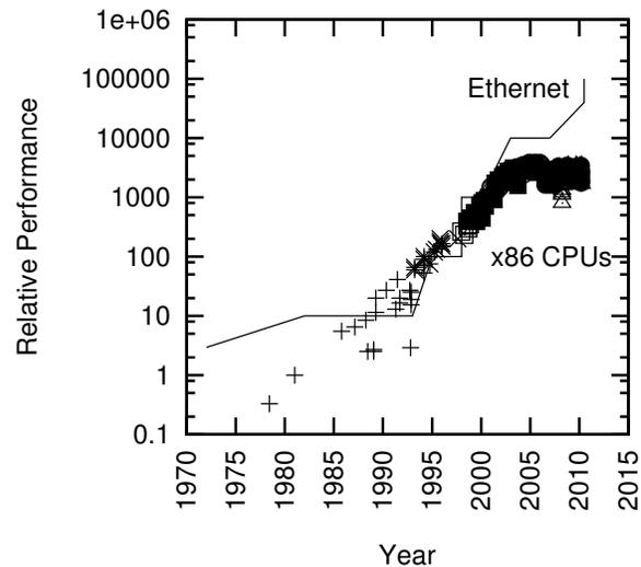
Figure 5.15: Ethernet Bandwidth vs. Intel x86 CPU Performance
