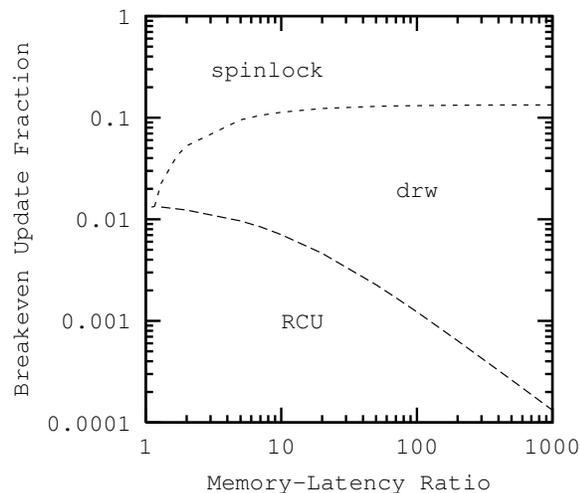
Figure 14.7: Breakevens vs.  $r$ ,  $\lambda$  Small, Four CPUs
