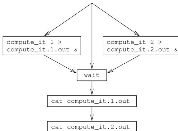
Figure 3.1: Execution Diagram for Parallel Shell Execution
