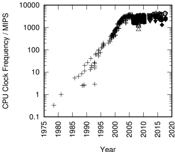
**Figure 2.1:** MIPS/Clock-Frequency Trend for Intel CPUs
