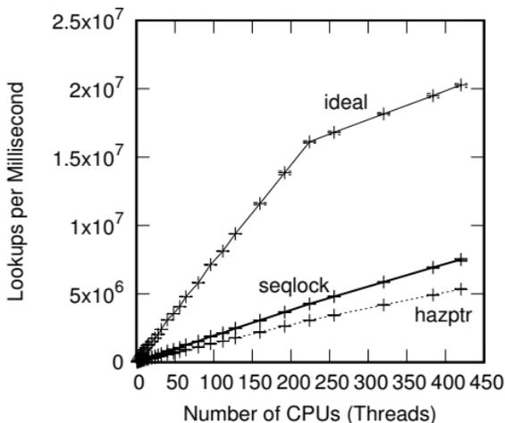
**Figure 9.5:** Pre-BSD Routing Table Protected by Sequence Locking
