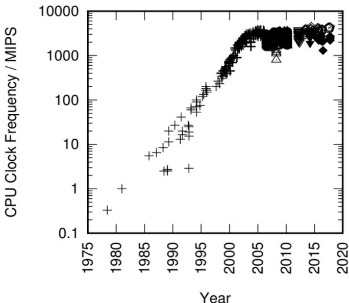
**Figure 6.11:** MIPS/Clock-Frequency Trend for Intel CPUs
