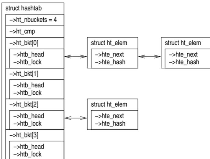
**Figure 10.1:** Hash-Table Data-Structure Diagram
