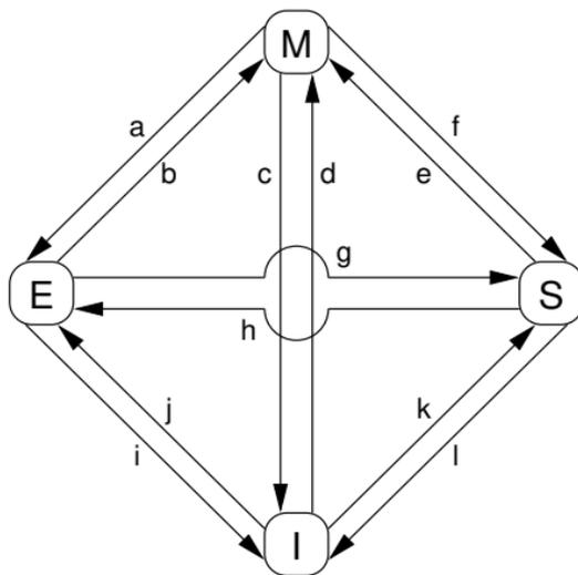
**Figure C.3:** MESI Cache-Coherency State Diagram
