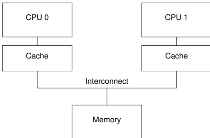
**Figure C.1:** Modern Computer System Cache Structure
