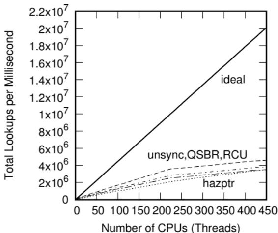
**Figure 10.9:** Read-Only RCU-Protected Hash-Table Performance For Schrödinger’s Zoo including QSBR and Unsynchronized, Linear Scale
