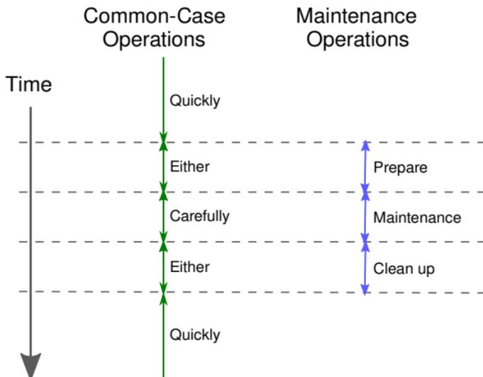
**Figure 9.24:** Phased State Change for Maintenance Operation
