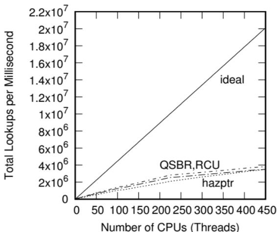
**Figure 10.8:** Read-Only RCU-Protected Hash-Table Performance For Schrödinger’s Zoo including QSBR, Linear Scale
