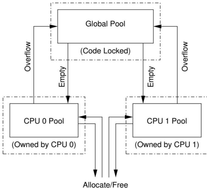
**Figure 6.19:** Allocator Cache Schematic
