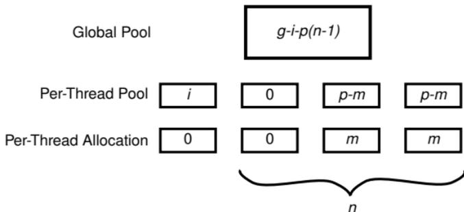
**Figure E.3:** Allocator Cache Run-Length Analysis
