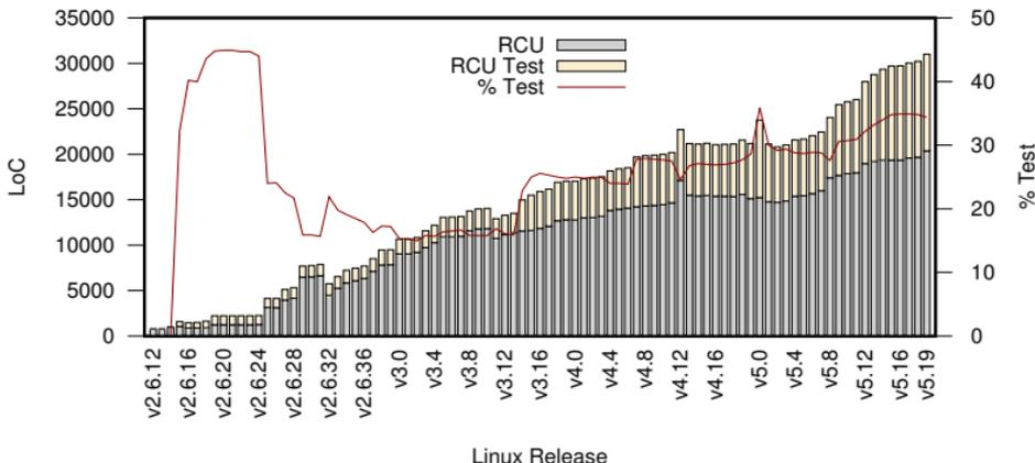
**Figure 12.4:** Linux-Kernel RCU Test Code
