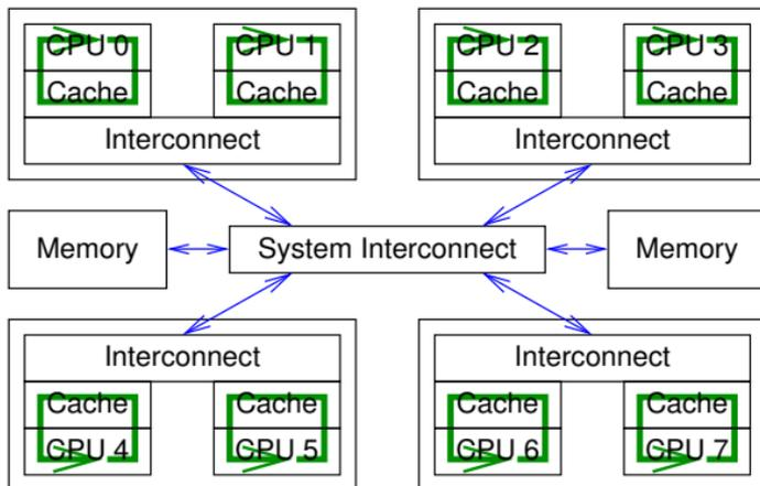
**Figure 5.4:** Data Flow For Per-Thread Increment
