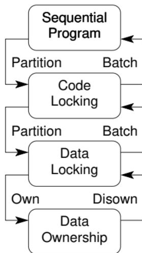
**Figure 6.10:** Design Patterns and Lock Granularity
