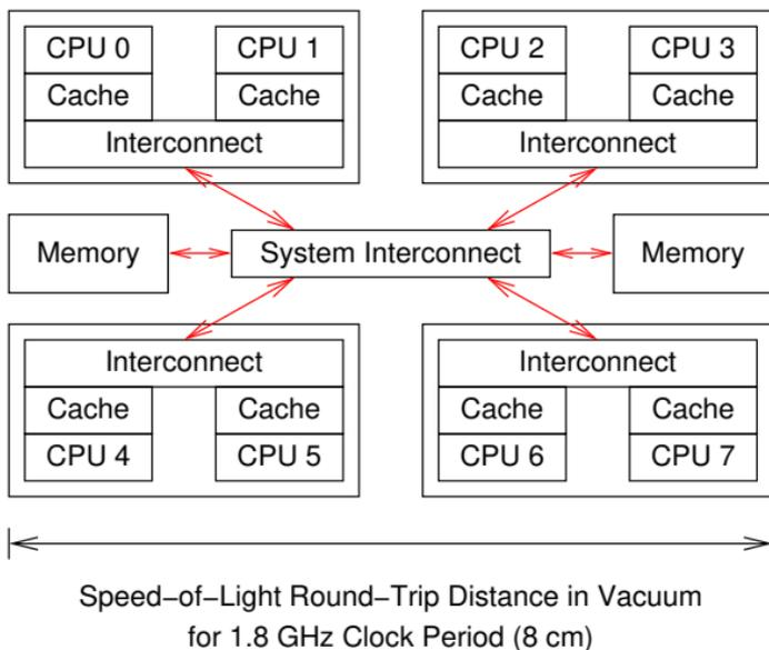
**Figure 3.10:** System Hardware Architecture
