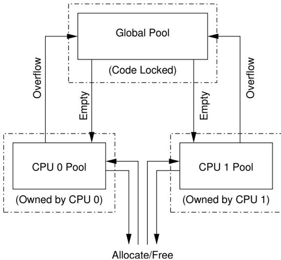
Figure 6.27: Allocator Cache Schematic
