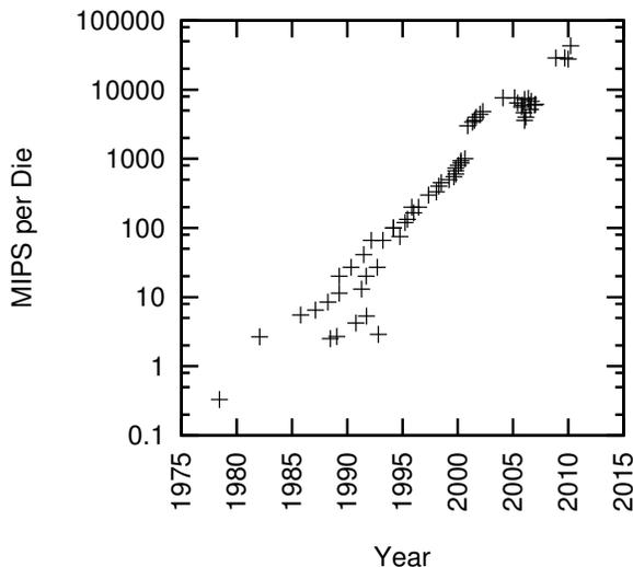
Figure 2.2: MIPS per Die for Intel CPUs
