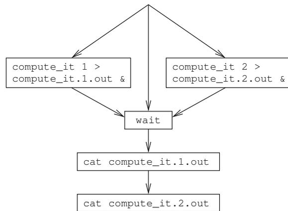
Figure 4.1: Execution Diagram for Parallel Shell Execution
